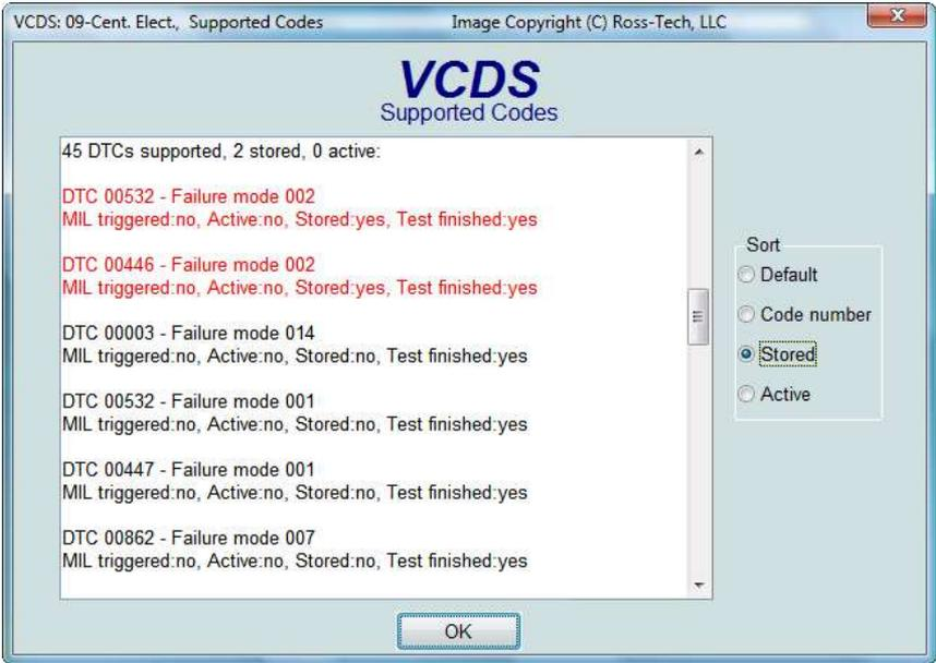
**Supported Codes function:** On the latest control modules which have this capability, VCDS can show all DTC and Failure Mode combinations which a control module is capable of detecting, including the current status of each.
