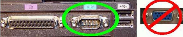
Observe the port we surrounded with the **GREEN** oval. Notice the 9 male pins? That's a Serial port. Observe the port circled and crossed in **RED**. Notice the 15 female pins? That is a Monitor port and will **not** work!
