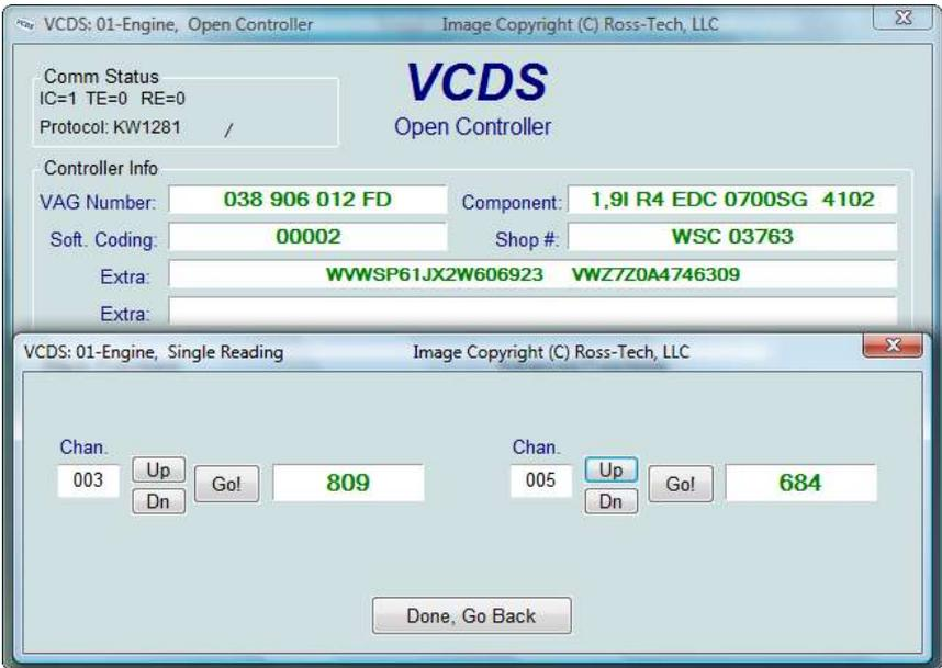
This function allows you to look at real-time data from control modules that support it. However, the data stream coming from the control module gives NO CLUE what the data means or how to scale it into real-world values.
