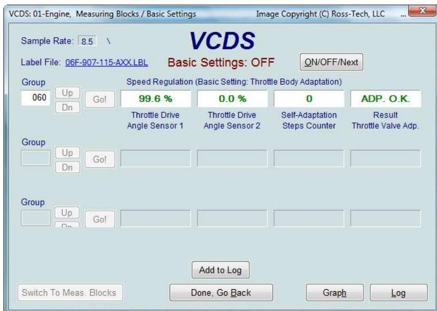
Basic Settings mode is very similar to Measuring Blocks and the contents of each display group is the same. The difference between the functions is that the Control Module may try to perform various calibrations while in Basic Settings mode.
