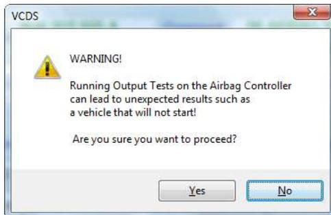
For example, in the VW Touareg, a specific procedure must be performed to be able to start the vehicle if Output Tests on the Airbag Controller have been performed.
