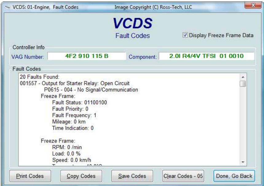
On this screen, VCDS shows you any DTCs (“Diagnostic Trouble Codes” or Fault Codes) present in the control module in which a communications session is currently active. VCDS shows the DTC numbers and also decodes each DTC into meaningful text.
