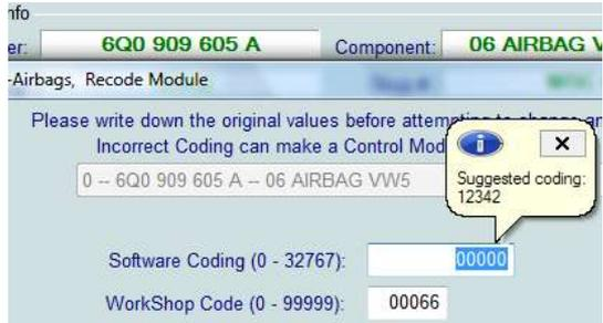
In cases where VCDS would offer Airbag module coding suggestions but cannot determine the Index automatically, VCDS gives you the ability to manually enter an Index (found on the Airbag controller sticker or work order) to get the suggested coding:
