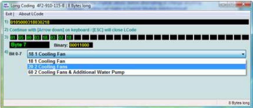
After making the desired changes in the Long Coding helper, closing that application (by using the [ESC] key on your keyboard or by clicking the Windows X box on the top right of the screen or clicking the Exit button on the top left of the screen) will send your new Coding value back to the Coding screen.
