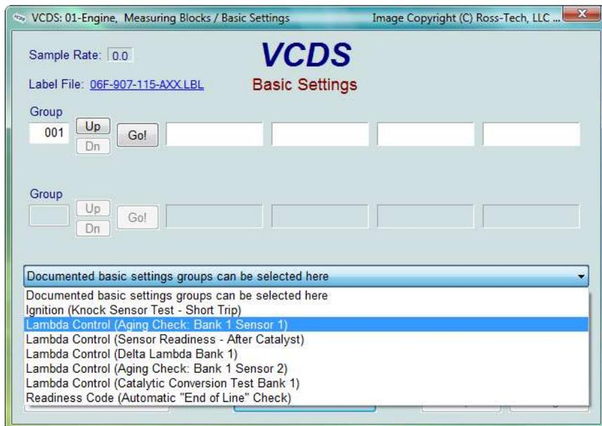
**Dual ECU's:** For vehicles with dual ECU's (like the Audi R8), the Basic Settings mode for both ECU's can be accessed simultaneously by addressing **[31 – Engine Other]**
