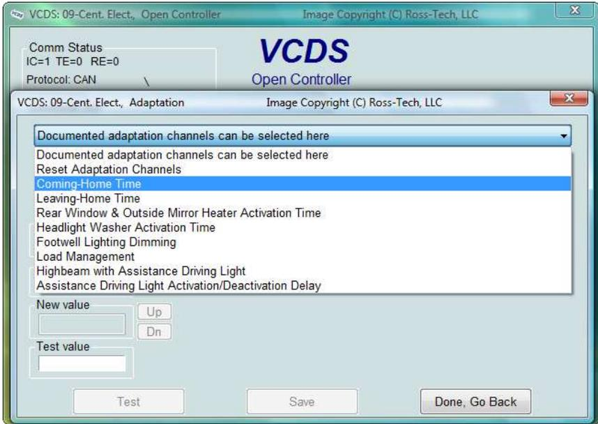
Once you have reached a channel of interest, you can use the **[Up]** and **[Dn]** buttons next to *New Value* to incrementally change the value. Or you can directly enter a *New Value* and click **[Test]**. This will tell the controller to temporarily use the new value so you can evaluate its effects.
