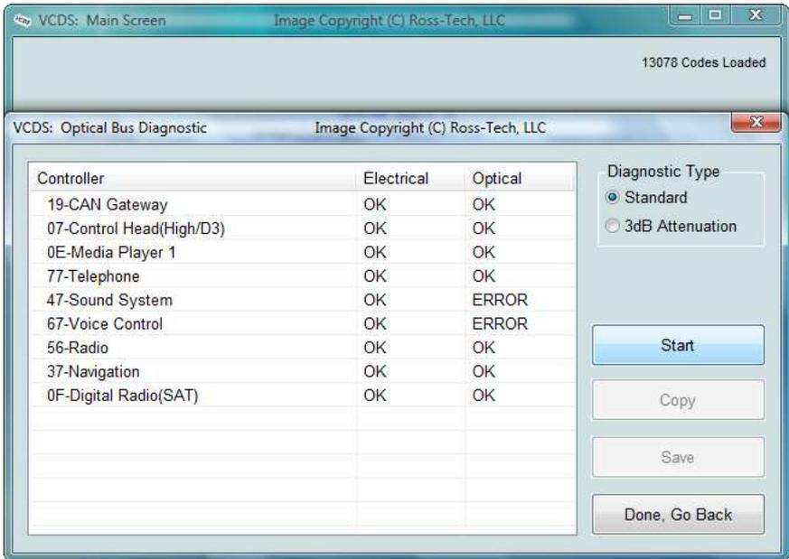
The **[Optical Bus Diagnostics]** function found in the Applications Screen is used on models with a MOST bus to narrow down the location of a break in the network. Many control modules will be completely inaccessible via conventional diagnostics if there's a break in the MOST bus.
