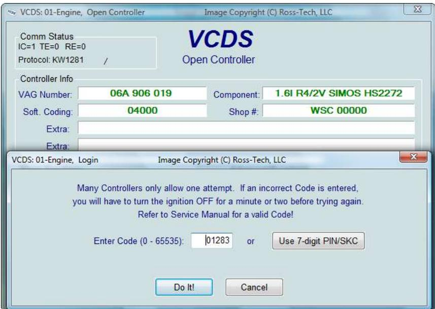
The Login Function must be used on some (but not all) Control Modules before you can Recode or change Adaptation values. On others, it "enables" certain features like cruise control. Valid Login codes can be found in the Factory Repair Manual for your car.
