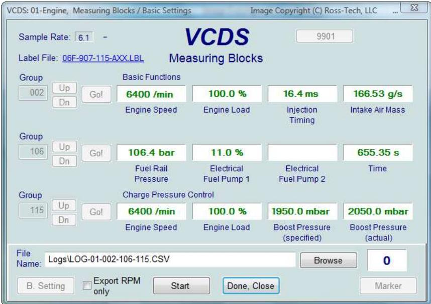
**Export RPM Only** when checked will record only RPM from the first field and will not record other fields. Also, this will only record RPM values that are non-zero. This feature can be useful if you are logging to output the file to a spreadsheet or other third party software
