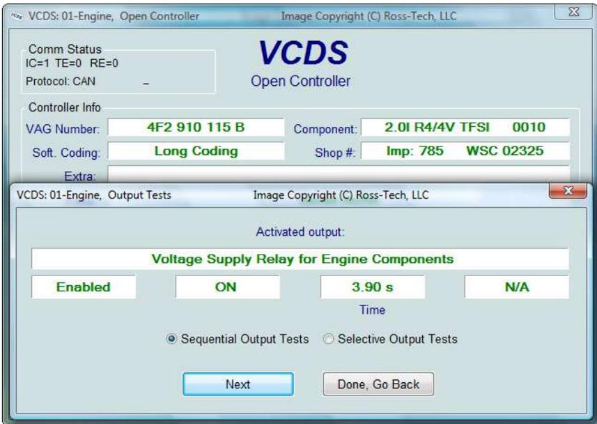
The Output Tests function is used to test a Control Module's Electrical Outputs (and the wiring that connects it to the various devices). Output Tests under KWP-2000/CAN/UDS includes simultaneous measuring data when available from the control module in question.
