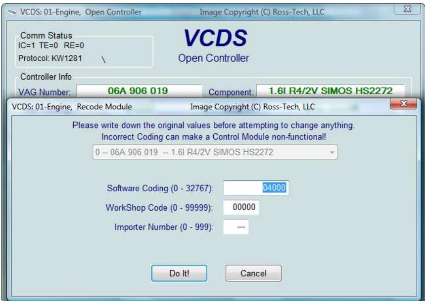
Recode is used to set various options in a Control Module. Note: Some Modules require a valid Login before you can re-code them.
