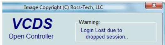
The most common cause of this is the use of an incorrect login code or a 7-digit PIN/SKC based on an incorrect Immobilizer ID or incorrect data entered in the 7-digit dialog. You will need to exit the Controller and do another Login.
