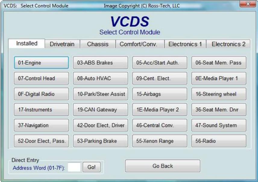
The various computers in the car are called "Control Modules" or "Controllers". On this screen, you select which Control Module you want to "talk" to. To establish communications with a particular Control Module, simply click on the appropriate button. For example, click on the button for **[01 – Engine]** to connect to the engine controller.
