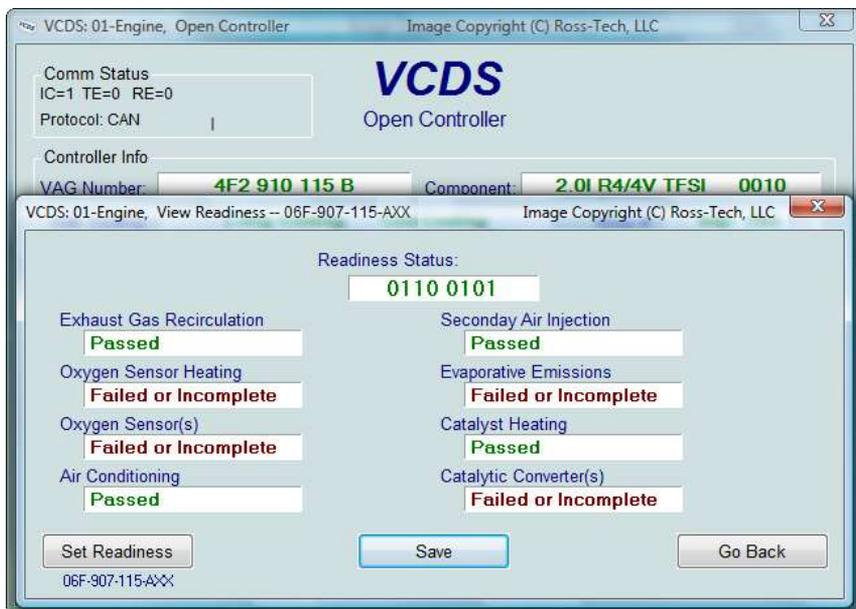
The Readiness Code is a set of 8 bits, each of which corresponds to one monitored emissions "system" in an OBD-II car. When all readiness bits show "Passed", it means that all systems have been checked and have passed the on-board tests. The Readiness screen shows name of script in title bar and under the [Set Readiness] button, or gives a reason why **[Set Readiness]** is disabled when that is the case.
