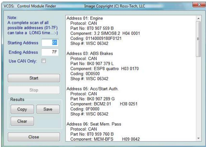
This function cycles through each possible address in the vehicle, finding each controller and reporting its Address, Name, Protocol, VAG Number, Component Number, Soft. Coding, and WorkShop Code.
