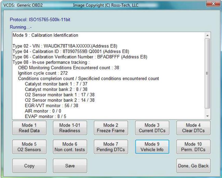
**Generic OBD-II functionality.** Because many of VW's recent factory repair manuals no longer have traditional 01-Engine "On Board Diagnostic" information and have replaced it with "Generic Scan Tool" data, this has become much more important than it was in the past. Click each of the Mode buttons to access each OBD-II function.
