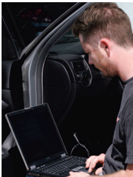
(above) It's easy to use, just install the software, plug VAG-COM into your laptop and connect it to your car
