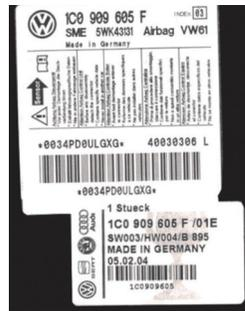
In cases where VCDS cannot automatically determine a coding suggestion, VCDS allows manual entry of an “Index” to get the suggested coding. See Figure 2. The Index is part of the “complete” part number for the new airbag controller. This part number and index can be found on the box of the new airbag controller, the invoice/order form for the airbag controller, or the stickers on the controller as shown in the adjacent photo.
