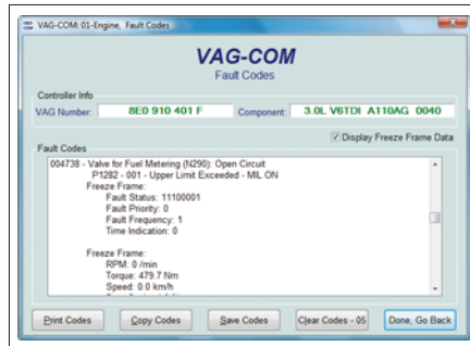
Stored fault codes are displayed with their explanation.
