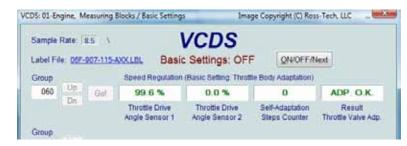
Procedure for performing the TBA on DBW cars that use KWP-2000 (typical of engine controllers in 2002+ Audi A4, VW Passat and Touareg)
