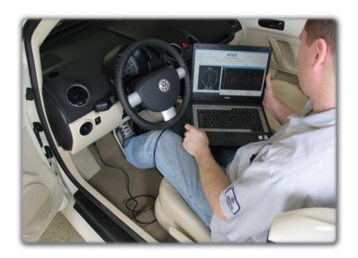
The extensive database in VCDS contains over 13,000 codes with helpful descriptions eliminating the need for you to look up the code. Included with the fault code number is a phrase describing the code and any stored Freeze Frame data.
